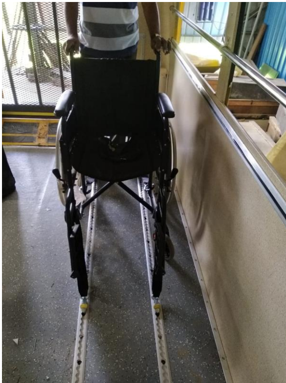
The wheel chair bus project- pics of both inside and out side the bus, wheel chair locking system in place, locking tracks the elevator
