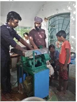
Over the summer we had laid a power cable from our switch box, we also fixed up the mill; however, the power needed required further work on power distribution at the school. Initially, when we ground Dhaniya and Turmericthe power tripped and with the support of FWE (Foundation for World Education) grant, we redid the input power lines at the school. We made herbal tooth powder and are currently using it during sleepovers at the school.
